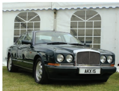
The Bentley Continental R was launched in 1992 with 360bhp, rising to 385bhp in 1997, which reduced the 0-60mph time from 6.6 to 6.3 seconds. Azure-style front seats with integral seatbelts were also added for the 1997 model year while the final 1998 models had curved pleats and partially rucked leather. They also gained a matrix grille, new alloys and restyled bumpers
